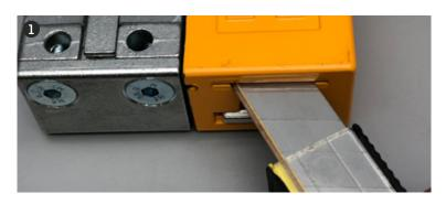
2 Unscrew the blade clamping plate with the Allen key (G), remove any dirt and change the blade.
