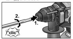
Check lock by pulling on the cutting accessory.
