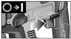
Press and hold down the trigger switch. The power tool trigger switch enables the speed or impact rate to be increased slowly to the maximum value.
