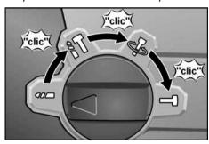
Setting rotary knob to the required operating mode:
