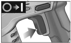
Press and hold down the switch. The power tool starts.
