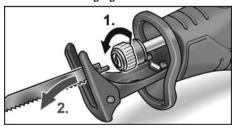
Release tool holder lock by turning anticlockwise and hold (1.).
