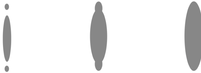
No atomizing air not enough atomizing air perfect atomizing air
