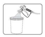
5. To fill the hose with the coating material, set the relief valve to spray and pull the gun trigger in parallel until material comes out of the gun. When filling the system, it is advantageous to turn the nozzle 180° (cleaning position) and hold the gun in the bucket. Secure the gun as soon as the system is filled.
