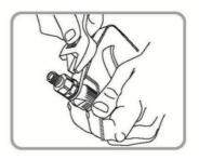
10. Remove holder and nozzle as well as filter
