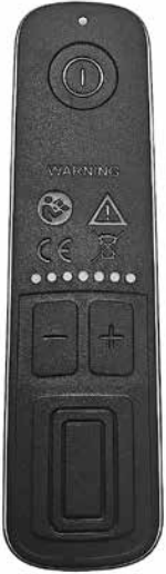
Power connected. Multi purpose led green.
